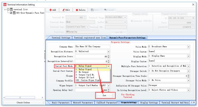
Setting Wiegand signal output and wiring. There is an example of connecting with the access control circuit board
